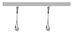
2. Install the other end of the hanging cable onto the fixed bracket of the lamp
