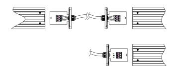
6. Install the end cap and complete the lamp installation
