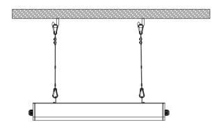
3. Install the lamp according to steps 1 and 2
